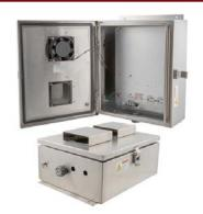
accuracy. The fan turns on when the internal temperature rises to 90° F (32° C) ±5° and turns off at 81° F (27° C) ±5°. Like the heaters, the cooling fan does not require the use of any of the AC outlets, leaving them all available for your equipment.
