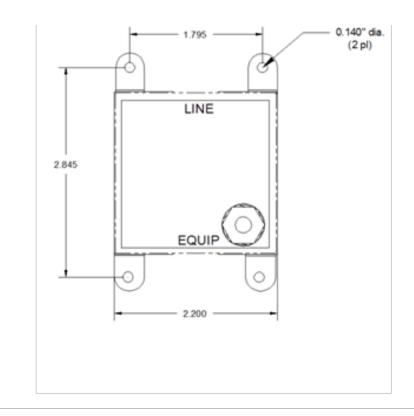
Equipment to be protected into the corresponding RJ-45 receptacle (EQUIP); connect the GND stud to the same system GND as the protected equipment using no smaller than a 14AWG wire.
